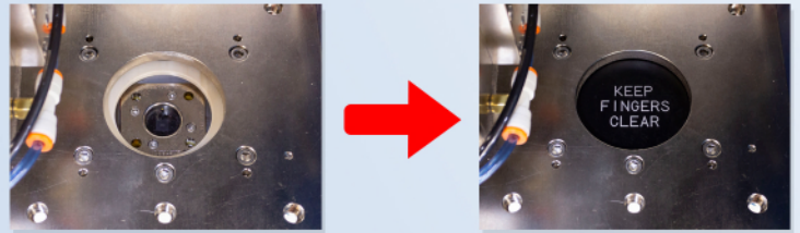
Shutter is open only during device removal/replacement
